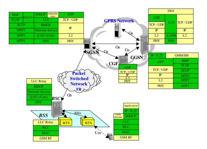
Figure 2 shows the protocols used in BTS, BSC, SGSN, GGSN, and mobile handsets:
