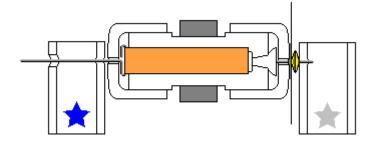
9. Glue the stand with the silver star to the board. Try to cover the corresponding star completely. Align the marks on the stand with the line on the board as shown below. Note that the star's position and the marks are approximate, sometimes you need to move the stands slightly to achieve the lowest friction. Keep in mind that super glue bonds instantly, so try to be as accurate as possible in these procedures.
