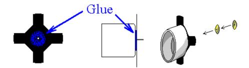
8. Insert the rotor into the stands marked with blue and silver stars as shown below. Hold the stands and test to see if rotor spins freely. Make final adjustments to the T-pin if necessary.
