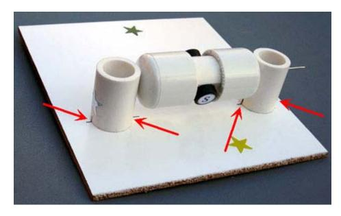
10. Insert the rotor into the stand marked with the blue star. Glue it to the board the same way as the first stand. Leave a gap of about 1/16" (1/32", or 0.8mm on each side) between the rotor and the stands. Test again to see if the rotor spins freely. At this time, or later, you may take the rubber plug and fix it as shown below. You can glue different things to the outer flat surface of the plug. Try to be accurate, redo this step if necessary.
