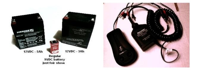
Only if you know what you are doing should you modify or change these devices. Here is the basic change I did for my own system. All you need is; a car charger that is 9vDC at 200-400ml Amp (about a 3rd of an amp) and use it as the power for the PhoneLynx. Incase power failure, the system will still work for weeks, even months (mine went about 120 days on fully charged 12vDC 5Ah Alarm Battery (about \$40-\$45) from my local battery store.
