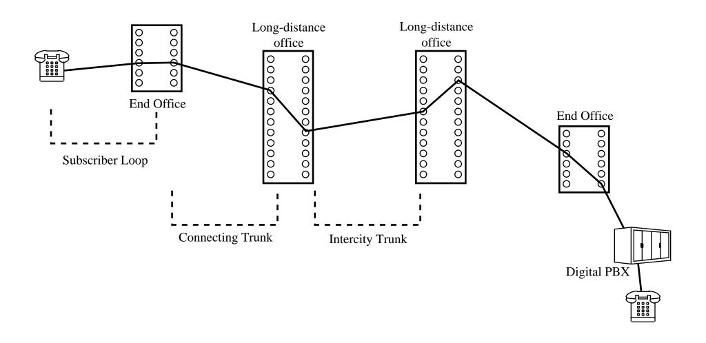
Figure 7.3 Public Circuit-Switching Network
