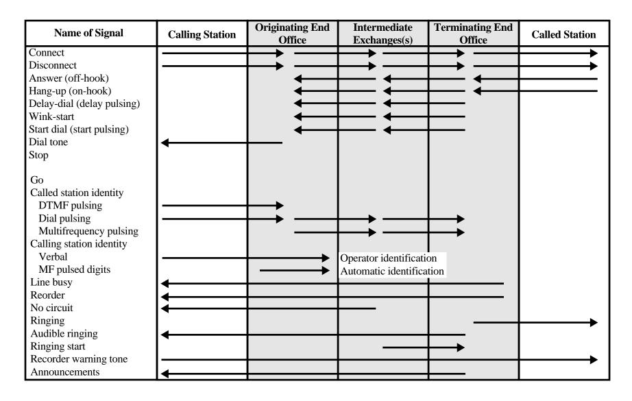
Note: A broken line indicates repetition of a signal at each office, whereas a solid line indicates direct transmittal through intermediate offices.
