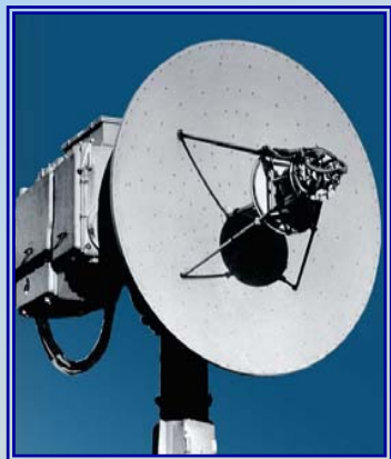
Telemetry information receiving post
