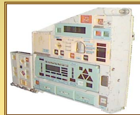
Tank system and mode control equipment
