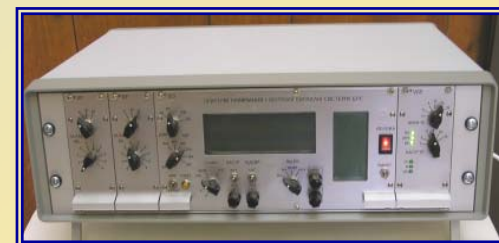
BRS-4 telemetry system radio signal receiving equipment
