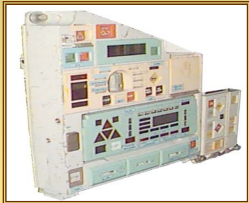
Tank system and mode control equipment
