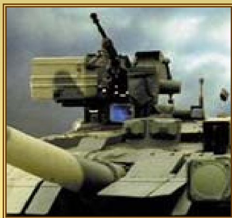
Tank with an antiaircraft mount
