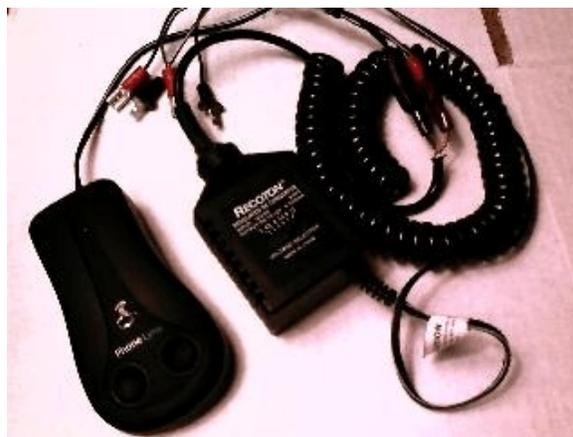
Only if you know what you are doing should you modify or change these devices. Here is the basic change I did for my own system. All you need is; a car charger that is 9vDC at 200-400ml Amp (about a 3rd of an amp) and use it as the power for the PhoneLynx. In case power failure, the system will still work for weeks, even months (mine went about 120 days on fully charged 12vDC 5Ah Alarm Battery (about \$40-\$45) from my local battery store.
