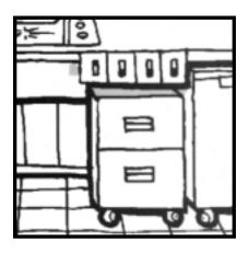
The controls of wall-mounted ovens should be located no higher than 40" above the floor so that persons in wheelchairs can reach them easily.
