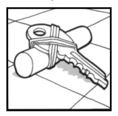
A lever arm welded or attached to an existing turn knob, may be an acceptable way to adapt your door locks.
