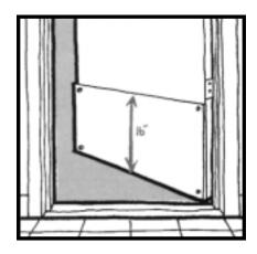
should extend from the floor surface up to a height of at least 10" and preferably 16". You can fasten plastic laminate, metal, and even hardwood kickplates to the door to provide protection. Kickplates should be as thin as possible so they won't reduce the clear door width opening.
