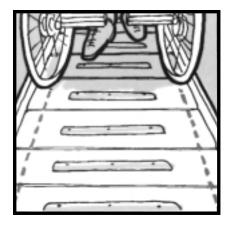
Broom-finished concrete is an excellent surface for exterior concrete ramps.
