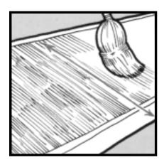
Make sure the broom strokes are perpendicular to the slope of the ramp.
