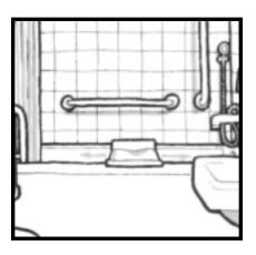
Several types of tub seats are available. Refer to the Resources chapter which begins on page 36 for manufacturers. You can also install a built-in tub seat, which will be more stable and safer than a removable seat. Be sure to carefully design this seat for drainage, so that water runs back into the tub and not out the side when you bathe.
