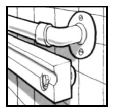
If you make rectangular wooden grab bars, allow closure between the thumb and fingers of your hand. This provides the best grip when you close your hand around the bar. The optimum diameter for grab bars is  $1\frac{1}{4}$ "- $1\frac{1}{2}$ " for adults. For a child or person with a very small hand, the ideal diameter is 1"-114". The distance between the wall and the grab bar should be 1½". A wider space can be dangerous if you slip and your elbow lodges between the wall and the bar. A narrower
