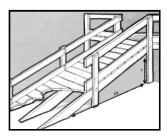
You can also use rolled roofing material. When properly tacked down, it provides a good non-slip surface for walking or wheeling.
