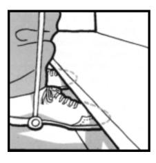
Nosings should be beveled, either by the insertion of a piece of wood or metal that will allow toes to slide up and over or by carpeting to slant the nosing projection.
