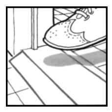
To remove a threshold, you must either cut or pry up and patch the flooring at wooden thresholds, or replace metal or masonry thresholds with others that have a lower profile. In some cases, you may be able to install a beveled ramp that abuts the edge of the threshold and eliminates the wheeling and tripping barrier.
