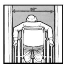
A swinging door is commonly available in a 3´ width, but 3´ doors are generally used only as front doors on
