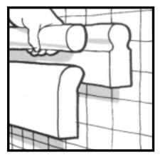
Handrails should be designed so that users can grip the rail between thumb and fingers. This "grasp-ability" or opposition is essential to the safety of users.
