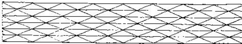
Fig. 12 Cylinder analyzed into rectangles and triangles
